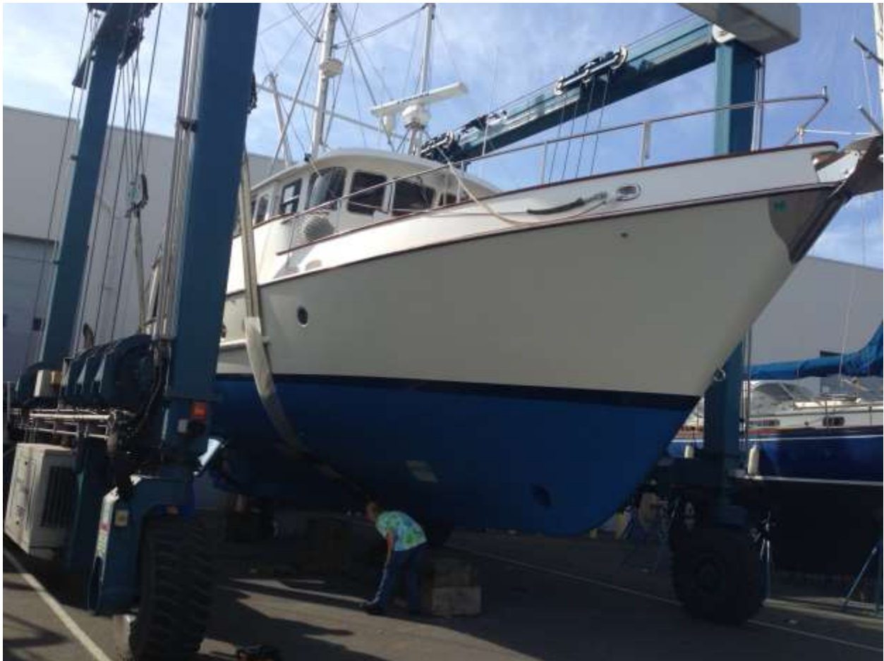
5 Blocking spots are painted over as the final preparation before launching.
