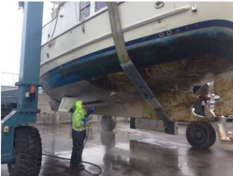
3 Pressure washing by the Port of Everett crew, one of her Naiad stabilizers is visible (we were surprised to learn they are not located symmetrically side to side)
